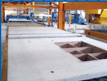
Greece, Prohellas Factory planning, multifunctional plant for girder slabs and double walls
