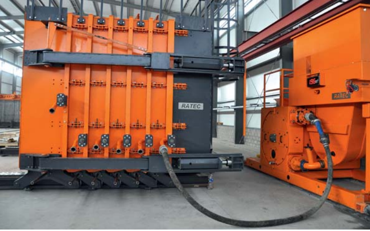
Battery formwork with movable pump car
