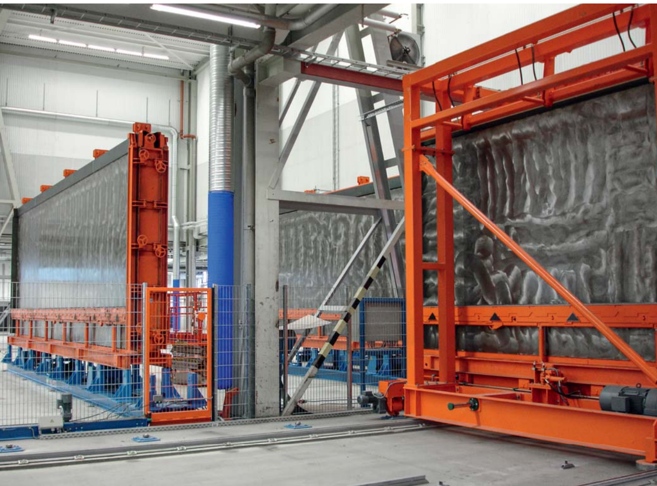
Planning of a battery production: Work stations with movable inner panels
