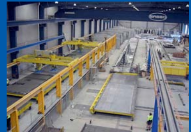
Australia, Austral Precast Factory planning, solid wall production
