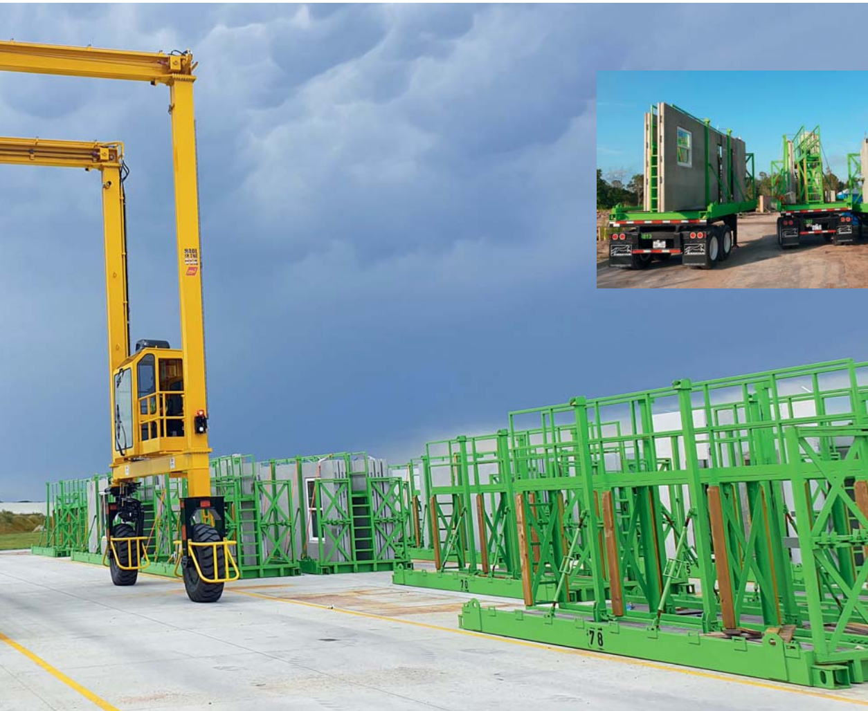
The handling in the outside area is done by a mobile gantry crane, which stores and retrieves the wall transport racks
