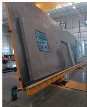
At the tilting station, the finished elements are lifted off and loaded onto transport frames
