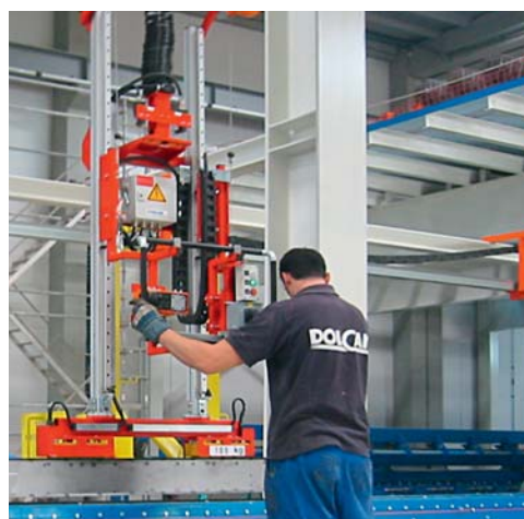
Suction turning frame in double wall production (left)
