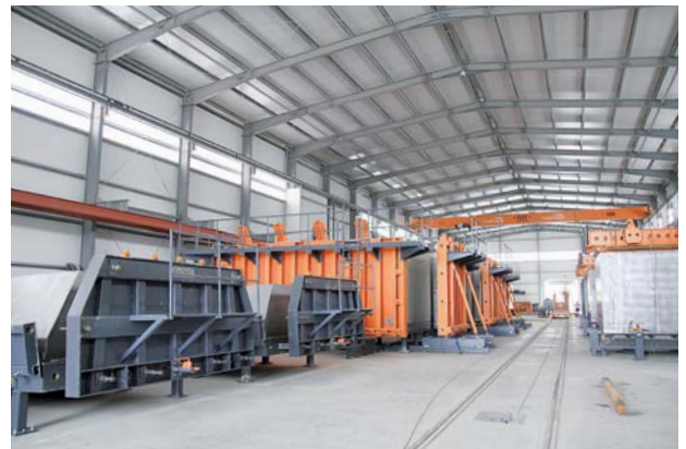
Module and roof formwork in the newly constructed plant in Ica
